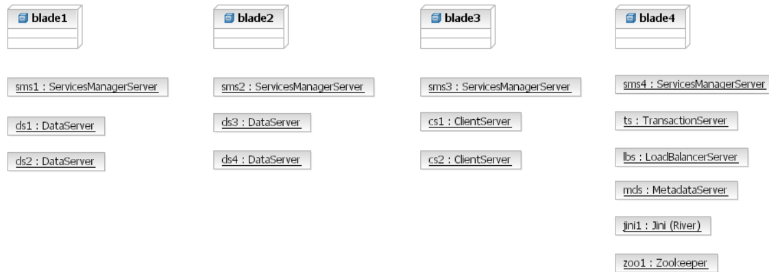
Figure 9 A sample deployment on a 4 node cluster. This is the minimum configuration for scale-out. Two machines are dedicated to data (blade1 and blade2). One machine is dedicated to client processing (blade3). The last machine is dedicated to various management services. In real world deployments, redundant instances would exist for critical services.
